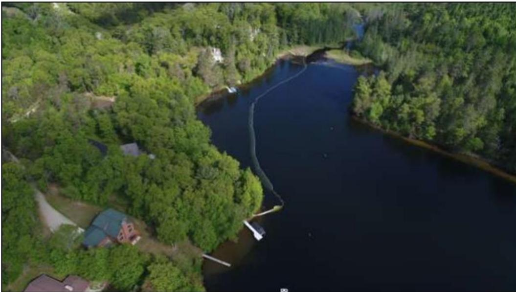
**Figure 20: Limno-curtain installed on Thunder Lake (photo from Marinette Co. LWCD)**
