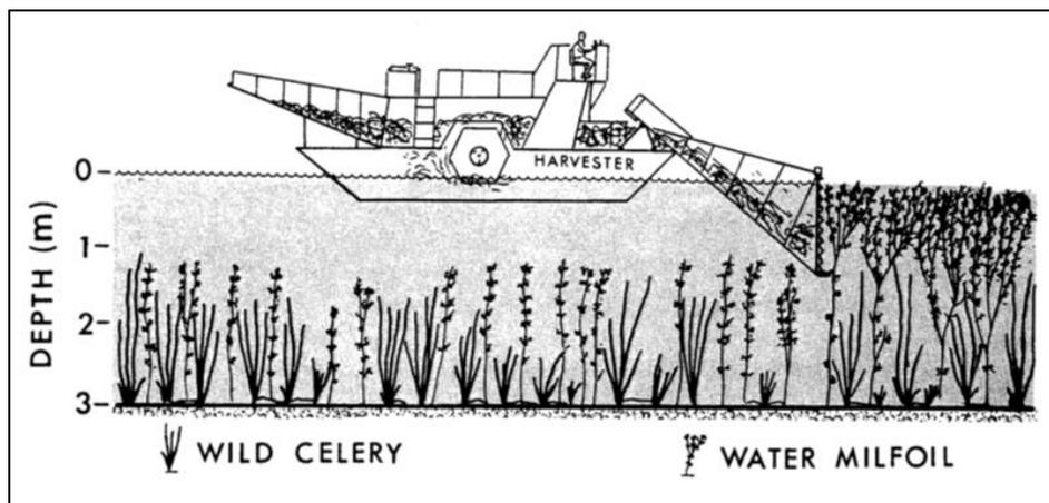
Figure 14: How a mechanical harvester works (Engle, 1987)
