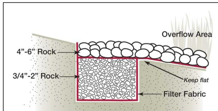
Figure 35: Rock Infiltration Set-up
