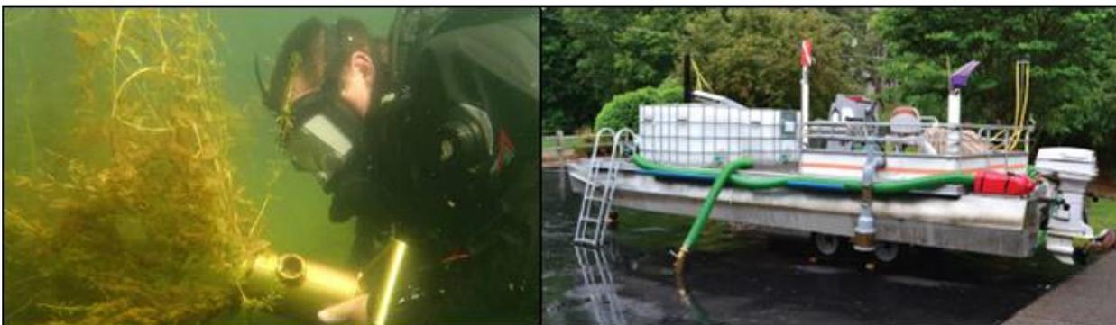
**Figure 13: DASH – Feeding EWM into the underwater Suction Hose (Marinette Co.); and a sample DASH Pontoon Boat (Beaver Dam Lake Management District)**
